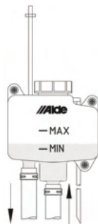
Fluid level in cold system
