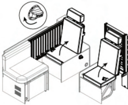
4. Lift up the bed slats on each bunk, ensuring these are restrained with the locking mechanism securely. Turn seat buckles anti clockwise to unlock the travel seats.
