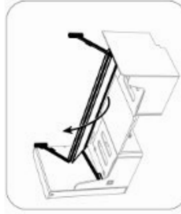
6 Position yourself in between the seats, lift the bottom of the fold-out bunk up and rotate folded base until horizontal. Ensuring the base stays folded.
