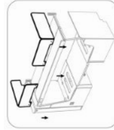
8 Locate then attach your drop in bunk supports, ensuring the metal plates are latched with the bunk frame
